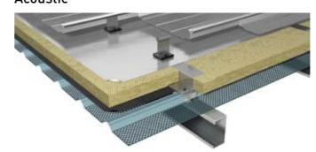
Build-up of perforated double skin roofing system
